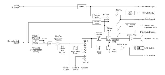
Figure 2.3 T885 Audio Processor Block Diagram
