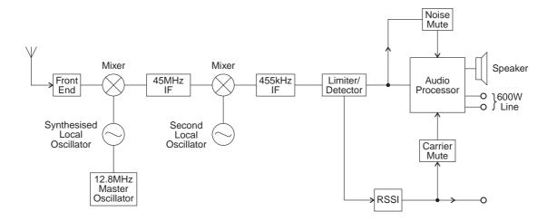
Figure 2.1 T885 High Level Block Diagram
