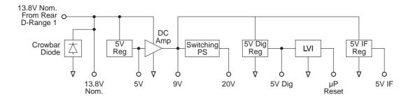
Figure 2.4 T885 Power Supply And Regulators Block Diagram
