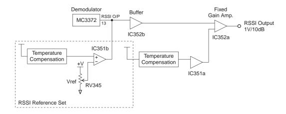
Figure 2.7 T885 RSSI Block Diagram
