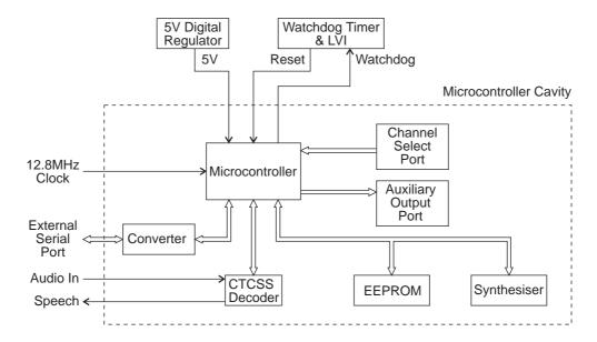
Figure 2.5 T885 Microcontroller Block Diagram
