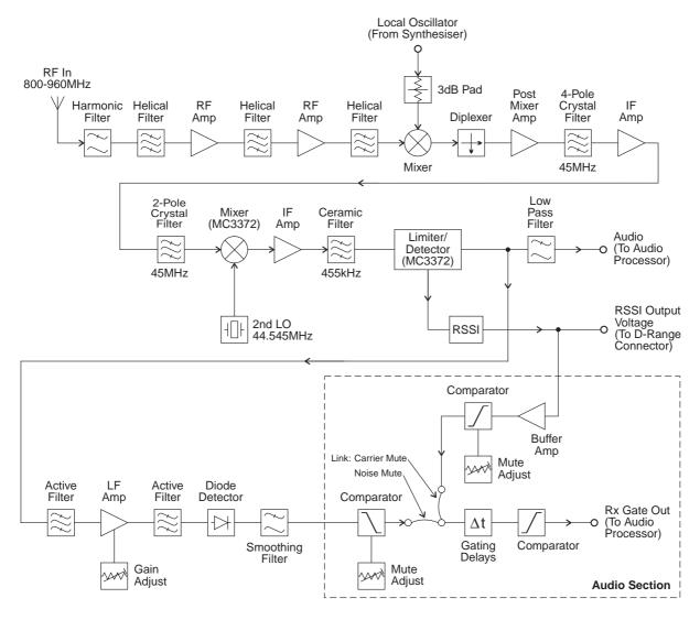
Figure 2.2 T885 Front End, IF and Mute Block Diagram
