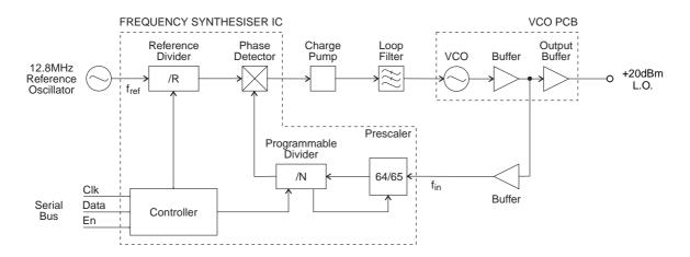
Figure 2.6 T885 Synthesiser Block Diagram
